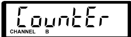
This display identifies the pulse counter (Channel B); it cannot be changed.
